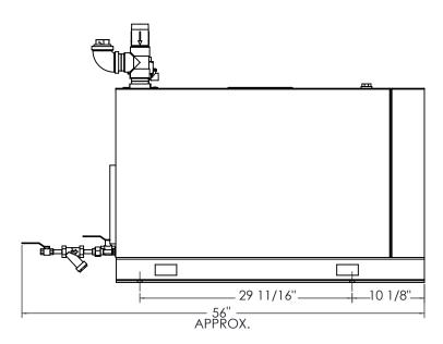
NOTE: PUMP MODULES ARE SHOWN WITH OPTIONAL EXTERNAL PIPING COMPONENTS FOR DIMENSIONAL PURPOSES.
