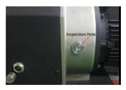
Inspection hole with G1" plug: Check the coupling and its insert, and fan through this hole regularly.
